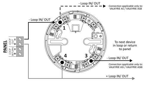
**NOTE:** Address programmed on switches 1-5 has an OFFSET of 94. For example if D.I.L. switches 1-5 are all set to OFF the actual sounder address, as read by the panel, will be 94.
